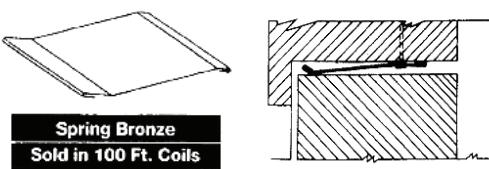
**C** An interlocking strip is best for the meeting rails. When the window is closed, the strips close off any air gaps. The sash lock pulls the meeting rails tight. (Courtesy of LC)
