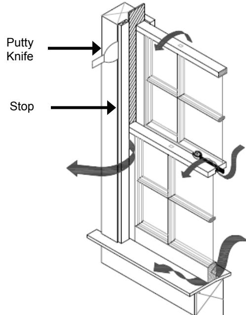
**Sticky Windows / Loose Windows:** Use a thin putty knife to slip behind the stop and lightly pry (you may need to run a knife along the edge on heavily painted trim). Simply loosening old paint will ease the motion, but some people apply furniture wax in the jamb channel to further reduce friction. Install weatherstripping to tighten.
