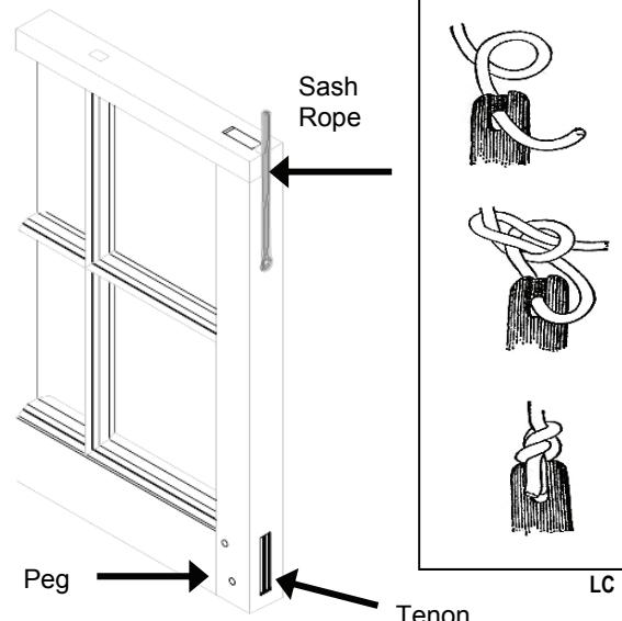
**Sash Cords and Weights:** A broken sash cord will require you to remove the window from the opening to access the sash pockets. Remove the stop then the sash, replace the cord and reattach it to the weight. A link to a good video demonstration can be found at: [www.preservationnation.org/issues/weatherization/windows](http://www.preservationnation.org/issues/weatherization/windows)
