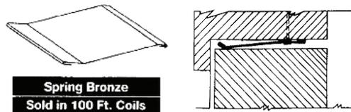
**C** An interlocking strip is best for the meeting rails. When the window is closed, the strips close off any air gaps. The sash lock pulls the meeting rails tight. (Courtesy of LC)
