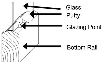
**Replacing Glazing and Putty:** Brush rabbets with oil-based primer prior to inserting the glass pane gently in place. Reinstall metal glazing points. Create a long strand of putty and press it along the muntin to make a beveled edge. Allow putty to cure before painting. Links to a video demonstration can be found at: [www.preservationnation.org/issues/weatherization/windows](http://www.preservationnation.org/issues/weatherization/windows)
